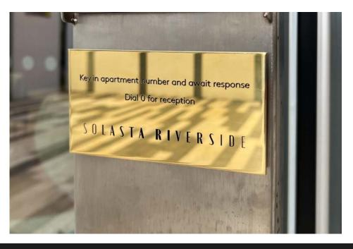
The 3mm thick brass panel features etched text and black infill paint. The face panel is bonded to a 3mm thick black foamex spacer and bonded to the substrate.
