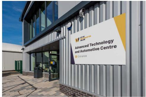
The 3mm thick router cut panel has been wet-sprayed, with vinyl lettering applied and a protective lacquer finish to preserve the sign detail.
