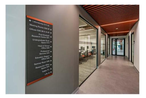
Thoughout the building we have fitted 3mm thick frosted lucite Jigsaw directory signage, with direct digital print to the face, with a high polish edge finish.
