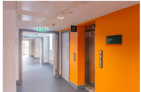
3mm thick frosted lucite directory boards feature high resolution direct digital print for excellent legibility. These are fixed to our patented Jigsaw directory system so that panels can be easily swapped without the need to replace the whole system.
