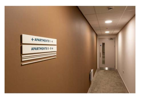
In the hallways we have provided Corian Cameo White wall mounted panel signs with engraved and resin infilled graphics in Evening Teal colour, bonded to 3mm black foamex spacers.
