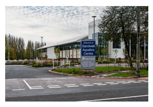
The external totem sign welcomes visitors to the centre. We've provided a fabricated aluminium totem, folded and dress welded with 2mm thick aluminium flat cut lettering and automotive grade paint.
