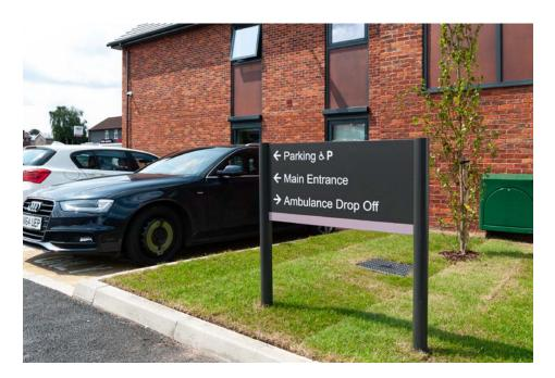
The external post and panel signs use aluminium planks with adhesive vinyls applied and extruded hollow aluminium legs.
