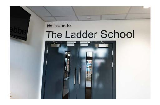
The internal cut letters in the reception area features 3mm thick, profile cut frosted lucite lettering with a high polish edge detail and a matt texture finish.
