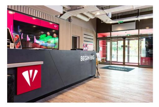
The bespoke, fabricated reception desk featured utilises a fabricated, illuminated brand sign with aluminium panels and 5mm acrylic graphics with cool white LED illumination.
