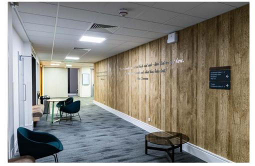
The quotation signage on the walls uses 3mm thick brushed stainless steel with glass bead blasted edging. We've mounted the signs with secure tape fixings.
