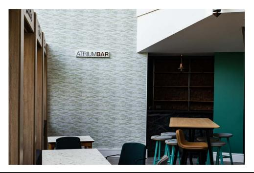
The atrium bar signage uses bespoke fabricated aluminium and Corten steel lettering with automotive grade paint finish. The letter faces and returns are dress welded and inlaid with LED module to provide ilumination.
