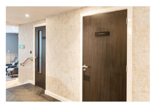
General door signs feature across the building, using 5mm thick matt black lucite panels and 3D Nitron Metallix copper effect foils.
