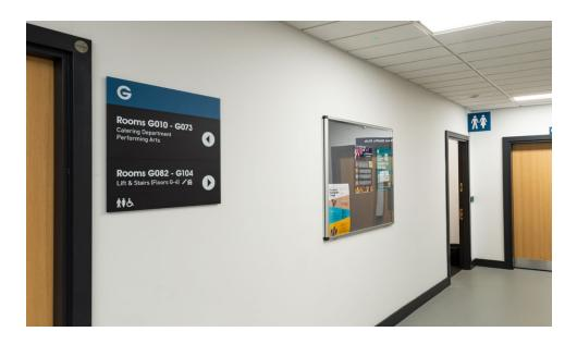
The corridors feature directory wayfinding signs using 4mm frosted lucite with high legibility direct digital print. The signs are mounted to the wall with our patented jigsaw system, allowing for easy change of panels.
