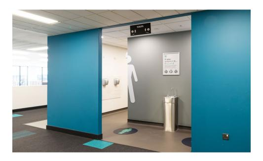
We've created 3mm frosted acrylic pictograms with a high polished edge and fixed to the walls to provide wayfinding for the facilities.
