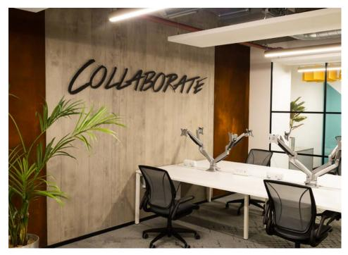
The 3mm cut letters in special font typeface is fixed directly to the wall with strong adhesive for security.
